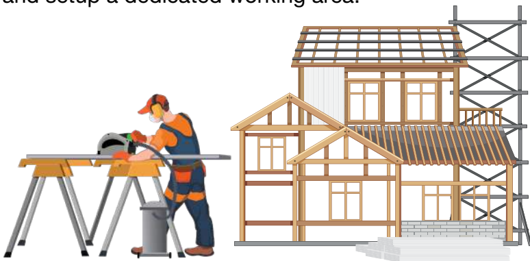
When using a power saw (e.g. track saw, circular saw or drop saw), dusts released must be controlled during work activity.
