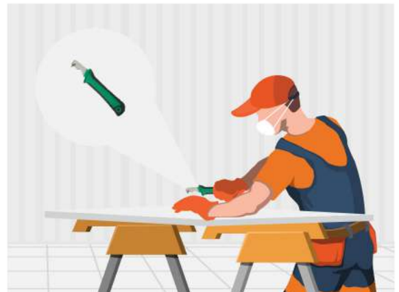
The best cutting technique involves using a score & snap knife, fibreshears or a hand guillotine.
